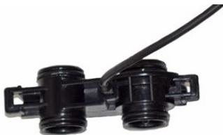
a) Choose which yoke (3/4" or 1") you wish to attach to the back end of the bypass. Remove the barrels (Figure 5) and apply a small amount of silicone lubricant to each of the O-rings (two on each barrel, four total) Push the barrels back into the bypass, and push the yoke onto the barrels. Attach the steel mounting clips on each side and screw in the two screws (Figure 6)
