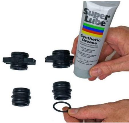
If the valve you are attaching the bypass to does not have a flow sensor, then it has the same type of barrels that are on the opposite side of the bypass. Take out the barrels and apply silicone grease to all four o-rings and push in the barrels and attach the bypass. See above picture for example of silicone grease and what an o-ring looks like.
