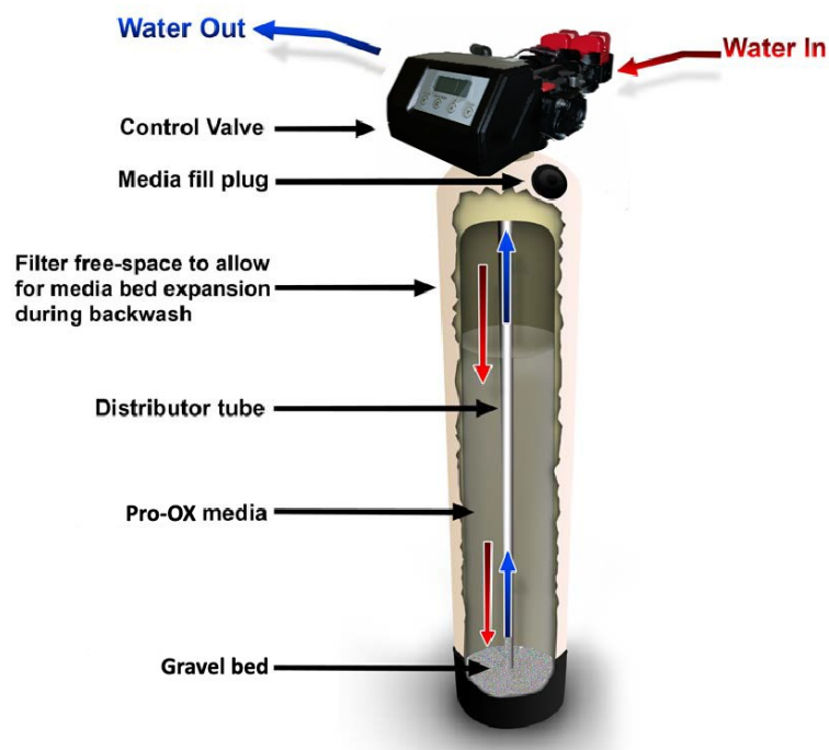
Fig. 1—Pro-OX Filter Tank Media Diagram
