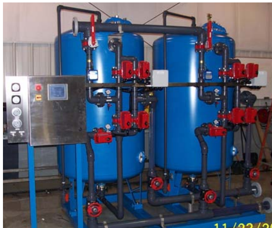
Use of E33 media in typical Modular and APU system installations.
