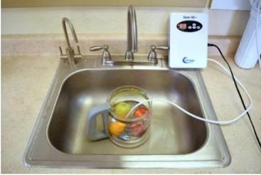
Place ozone diffuser stone in glass carafe or large bowl, add 1 - 2 gallons of water and fruits or vegetables or meats to be sanitized. Run ozone into container for 5 minutes. Let sit for 10 to 20 minutes, then rinse with disinfected water.
