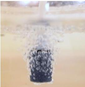
Fill 1 gallon glass or plastic jug with water and place ozone diffuser stone at the bottom of the jug. Run ozone for 3 minutes. Place lid on jug and let sit for 15 to 30 minutes.
