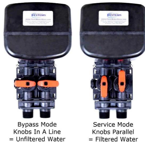
Fig 5: 5900e Bypass and Service Positions
