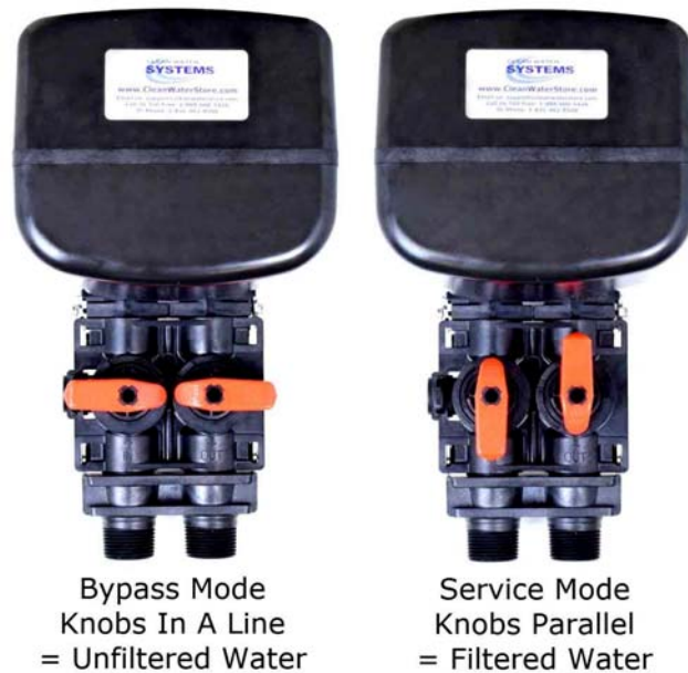
Fig 4 5900 Bypass/Service Mode Knob Positions
