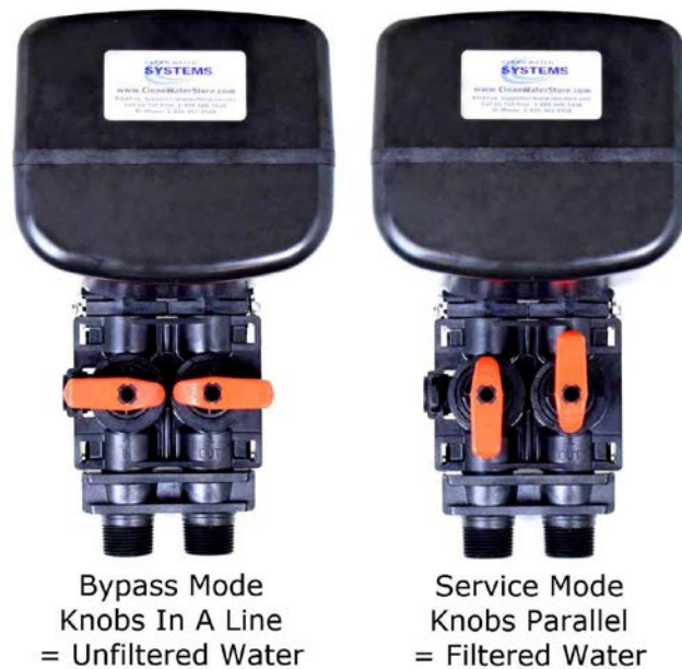
Fig 4: 5900e Bypass/Service Positions
