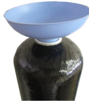
2. Add the filter gravel that came with your order. You will want the gravel to cover the bottom distributor screen before adding the Calcite media.
