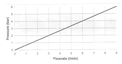
Capacity 4.5 l/min. (1.18 GPM) at 3 bar (43.5 PSI) and 20 °C (68 °F)
