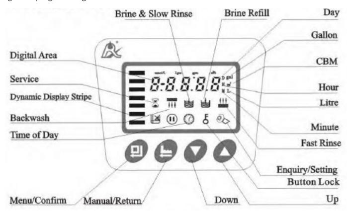
**IMPORTANT:** Before any operation, the valve menu must be unlocked. If the button lock indicator is displayed, press and hold both the Up and Down buttons for 5 seconds. A sound will indicate the menu is unlocked. The menu will re-lock automatically after 1 minute of inactivity.
