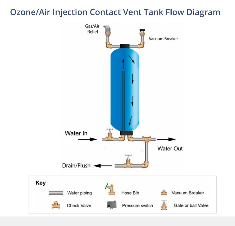
NOTE: Do not attach rigid copper or steel pipe to tank without using flexible connectors. Use flex lines on the IN and OUT if using rigid copper or steel piping. Contact tank may expand and contract during changes in line pressure, causing damage to tank if installed using rigid piping with no ability to flex slightly. We have flex lines if you need to order some.
