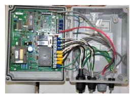
CE 1 Electronic Control Box (showing red lead from flow switch)
