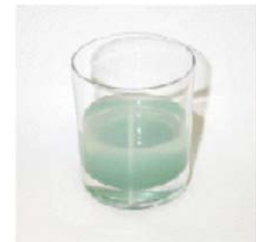
Blue water from a plumbing system with corroding copper pipe. Blue stains and blue water are an indication of copper corrosion.
