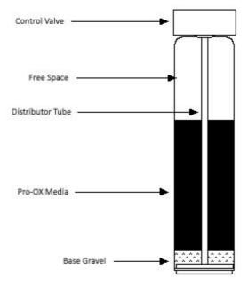
Fig. 2—Typical Pro-OX Iron Filter Installation
