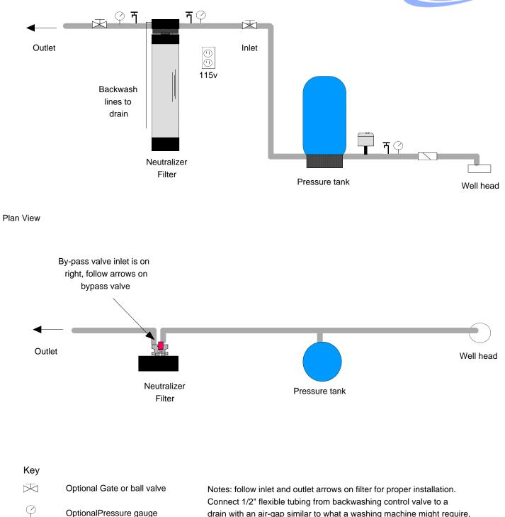
ሻ Optional Hose bib drain with an air-gap similar to what a washing machine might require, such as 1 1/2" ABS with a p-trap and vent or to other type of drain. Follow all local plumbing and electrical codes.
