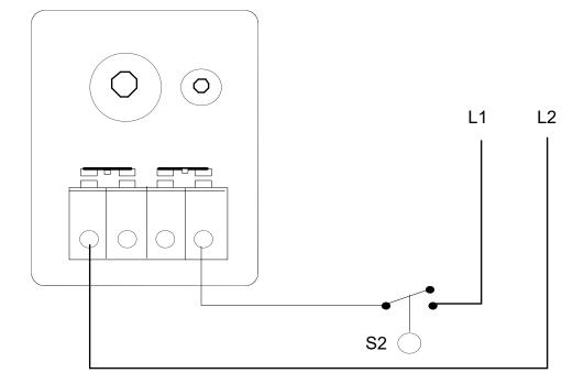
Typical pressure switch wiring with "normally points closed when floating" type float switch:
