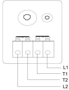
Typical pressure switch wiring: Load side (T1, T2) to pump motor; Line side L1, L2, to power in. This type of wiring directly controls pump motor. 2. Pressure Switch With Four Wires Direct control of pump motor with pressure switch 220v, ph1, with protection by lower float switch in storage tank
