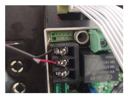
5.) Note: If you are hooking up multiple systems, use additional supplied wire to connect (daisy chain) the control valves together using the same middle common and normally open locations.
