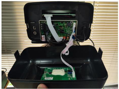
3.) Remove front cover and knock out plug. Run smaller control wire through port and secure using cable restraint.
