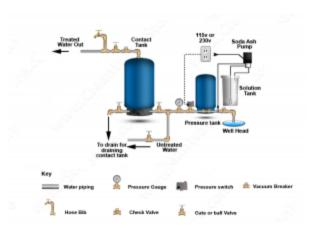
Note your water may not need 150 ppm of the 10% soda ash solution, it might only need 50 ppm to bring up the pH to the 7.0-8.0 range, but you will be able to know immediately after turning on the system by checking the pH.
