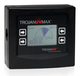
The optional COMMcenter displays dose in real-time and can monitor up to 9 UV systems - that's up to 270gpm!
