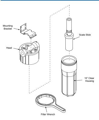
Scale Inhibitor System includes Scale Stick, 10" Scale Stick Clear Housing, Head, Mounting Bracket, and Filter Wrench.
