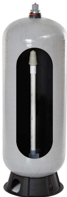
The new WellMate<sup>®</sup> BAFFLE tank from Pentair promotes uniform mixing and improved contact time in order to meet a .3 minimum baffle factor, as set by many health agencies. The distribution system in our tank provides for water to enter the bottom of the tank, distribute at the top of the tank, and exit at the bottom of the tank, providing maximum contact time.
