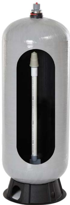
The new WellMate<sup>®</sup> BAFFLE tank from Pentair promotes uniform mixing and improved contact time in order to meet a .3 minimum baffle factor, as set by many health agencies. The distribution system in our tank provides for water to enter the bottom of the tank, distribute at the top of the tank, and exit at the bottom of the tank, providing maximum contact time.
