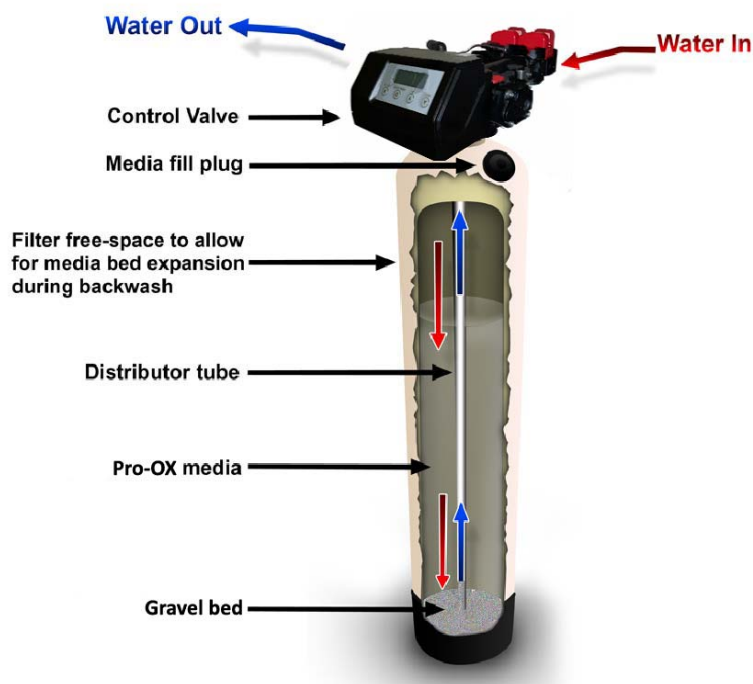
Fig. 1—Pro-OX Filter Tank Media Diagram
