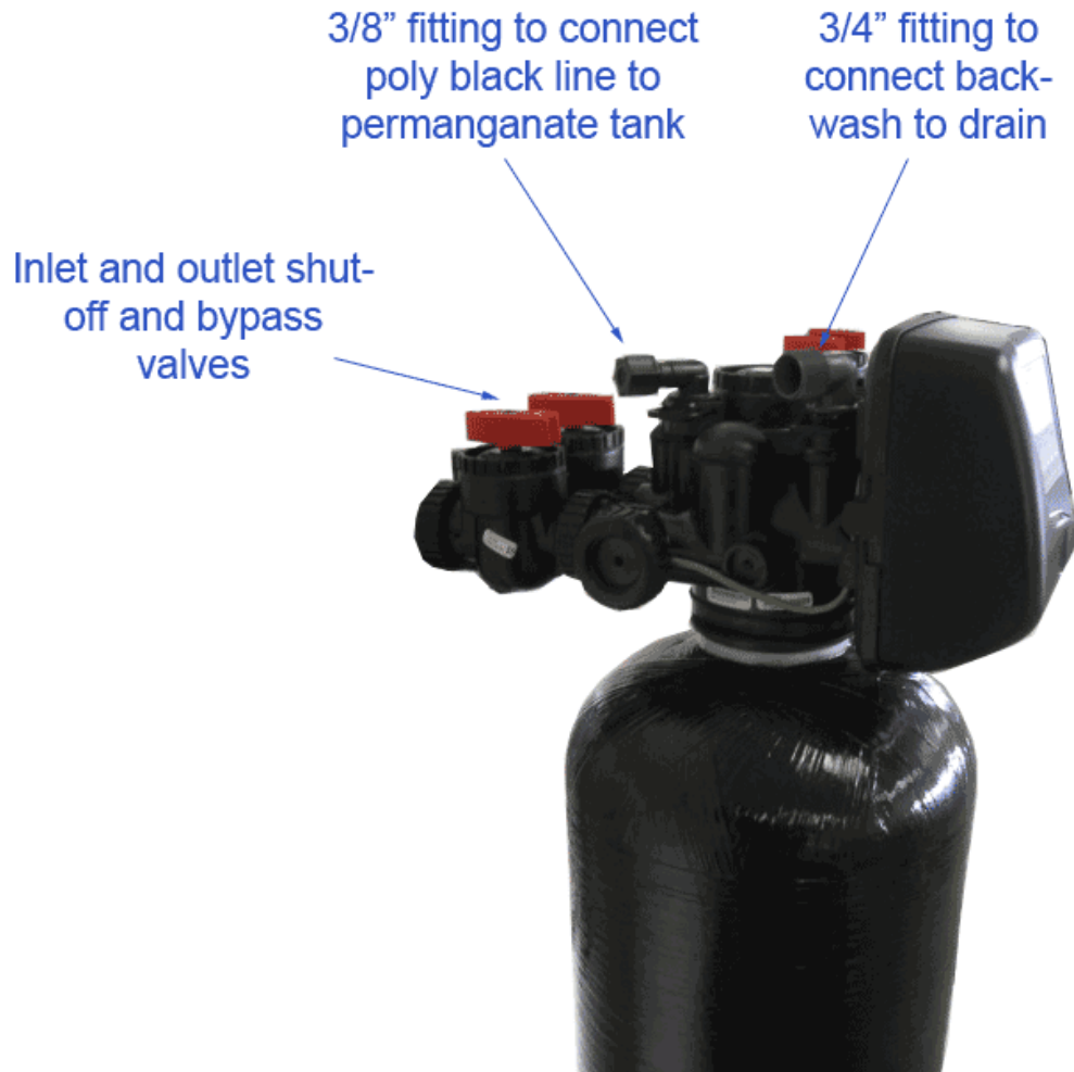
Fig 2: Clack WS1 Greensand Iron Filter
